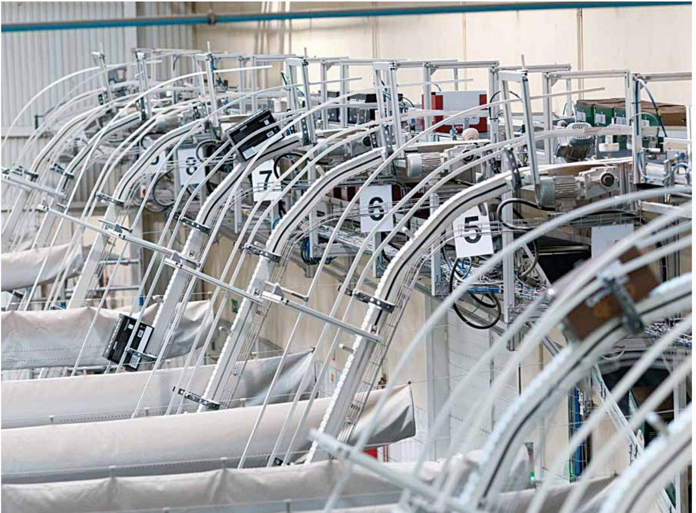
On traditional systems, large or bulky products require curves with a large radius and high friction coefficient. Rexroth takes a different approach: curves with ball bearings generate rolling friction. This means less friction and wear, as well as lower energy requirements and higher loads.
