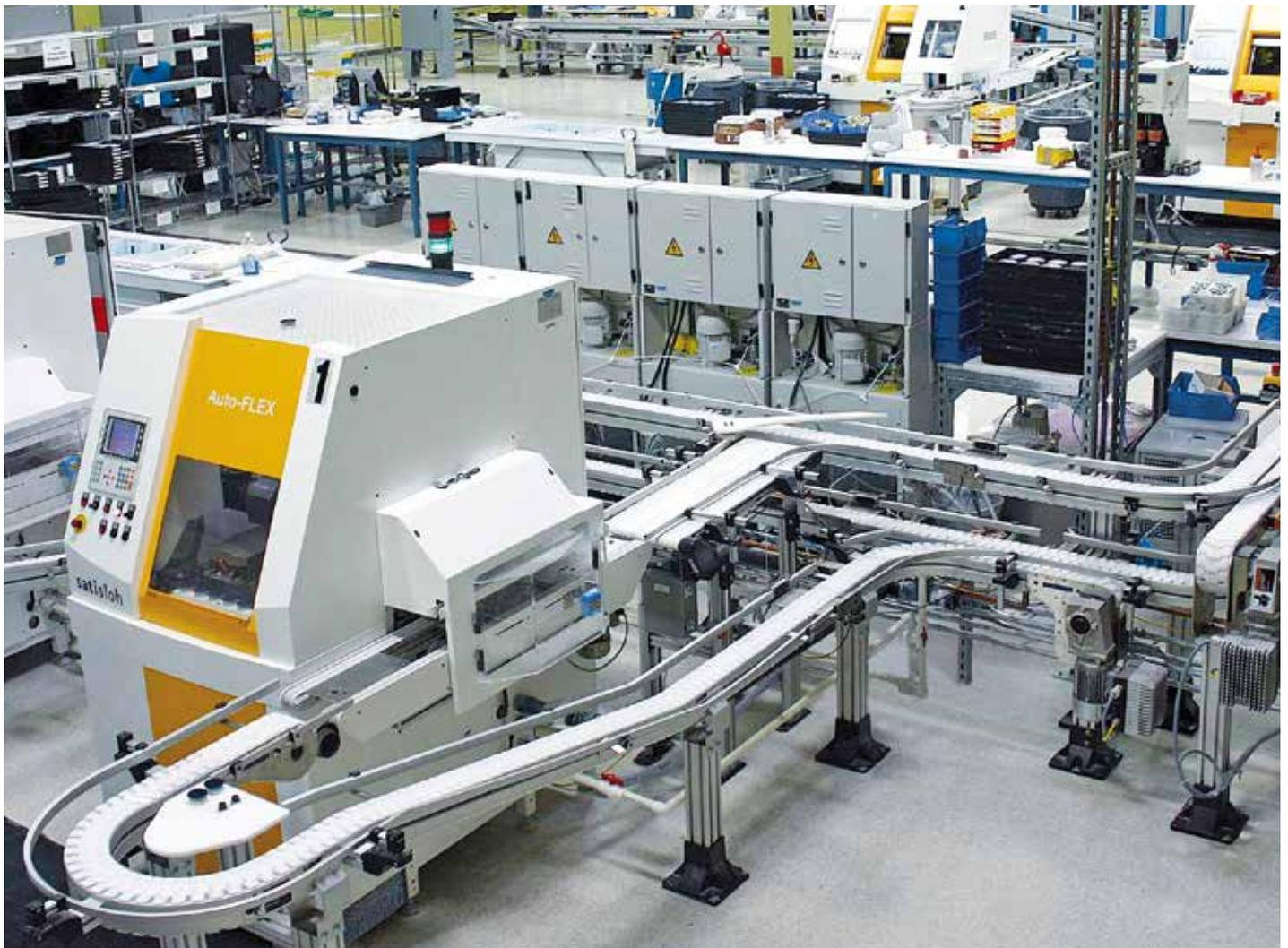
Even in nearly chip-free and modern machine tool linking, VarioFlow *plus* convinces with its use of largely media-resistant components. Application in the lower load range is inexpensive and economic compared to previous, heavy systems.
